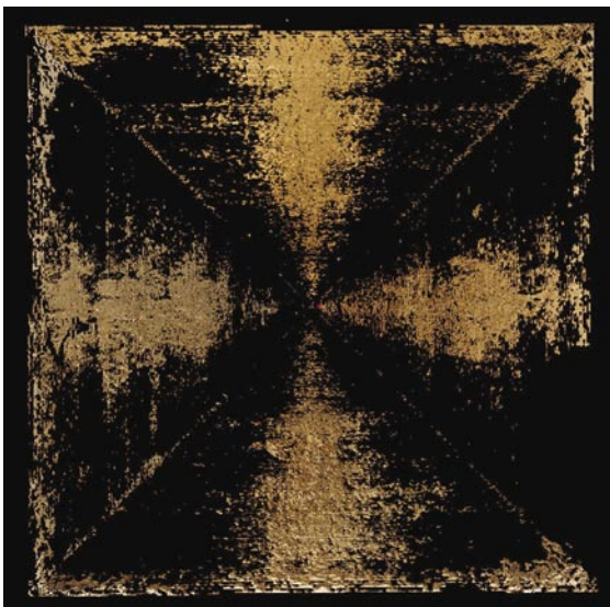
Fig. 9: Anomalous areas of the Cheops Pyramid visualized by color coded deviation from the ideal plane of the west face and as a horizontal projection showing anomalies within each side.
