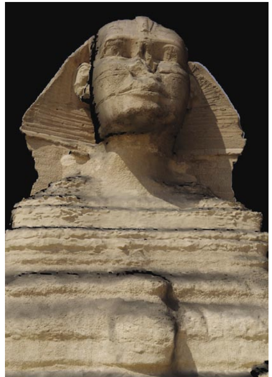
Fig. 6: Triangulated point cloud of a single scan textured with the acquired digital images.
