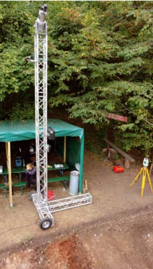
Arranging the 3D Laser Scanner for the record of complex surfaces uncovered during the excavation of the Iron Age workshops at Schwarzenbach-Burg.
