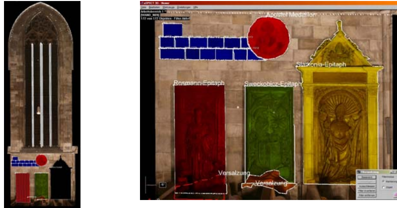
Fig. 10. Detail of 3D Mapping / Damage-Recording of wall element "N09"
