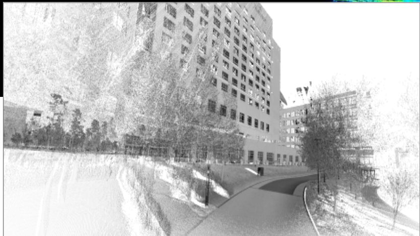
Data acquired with the RIEGL VMX-250 Mobile Laser Scanning System is visualized as point clouds in different view types, e.g., color coded reflectance (above) or grey scale coded reflectance (right).
